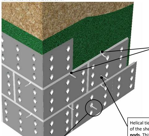
SIP panels do not have main support timbers so the tie can be placed in any suitable position along the length of the SureCav panel.
